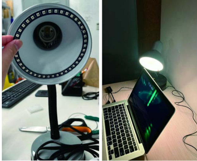
Figure 8: The modified desk lamp used in the control group, equipped with the identical RGB LED ring as embedded in the Light Everywhere prototype.
