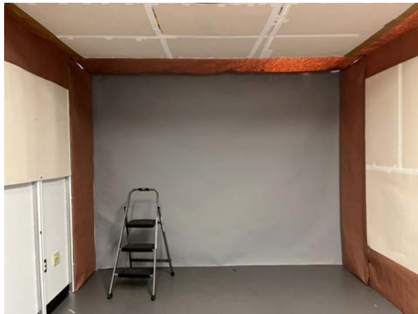
Figure 6: The “living room” being constructed in our laboratory. The white areas are the embedded magnetic sheets.
