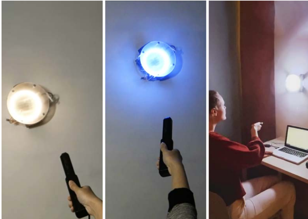
Figure 1: Light Everywhere , a robotic light fixture that climbs across walls and ceilings.
